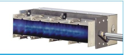
**FIGURE 2.** In a low  $NO_x$  line-style burner, the cut-outs and holes in the mixing plates cause the air and fuel to mix thoroughly, ensuring as uniform combustion as possible.
