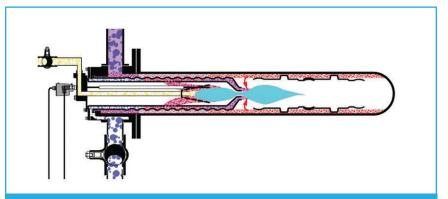
**FIGURE 3.** For applications requiring higher temperatures, one common method to reduce NO<sub>x</sub> is through the use of flue-gas recirculation (FGR), as shown with the red arrows in this cutaway of a self-recuperative burner in a radiant tube.
