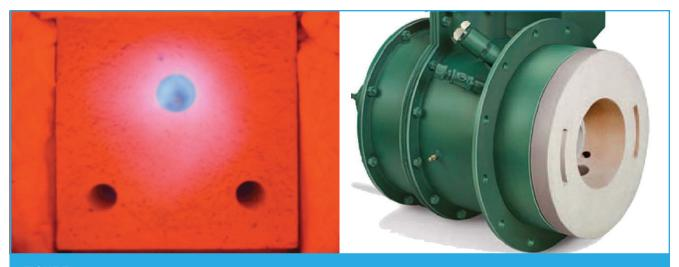
**FIGURE 4.** The telltale sign of a burner designed for staged combustion is an extra set of holes or slots for the secondary stream to travel through and into the combustion chamber. Here, two types of air staging are shown: holes on the left, slots on the right.
