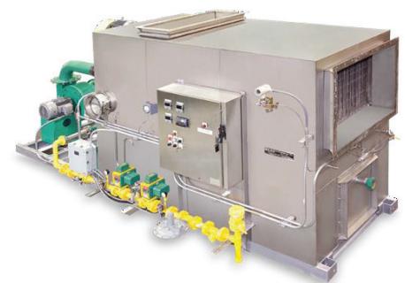
Figure 9: An indirect air heater, which combines an ultra-low NOx burner with a sinusoidal-plate heat exchanger can provide low emissions and effective process air heating.
