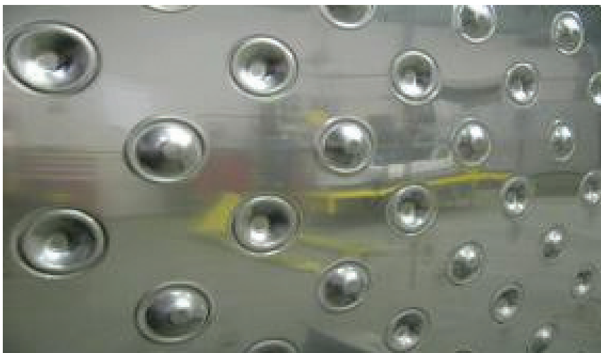
Figure 4a: Example of Dimple Plate Heat Exchanger
