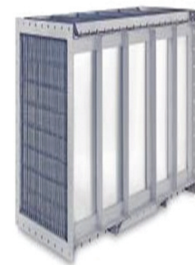
Figure 3: Plate-type heat exchangers use a series of nested plates to allow the exchange of heat between the two media without the two air streams coming into contact with each other.
