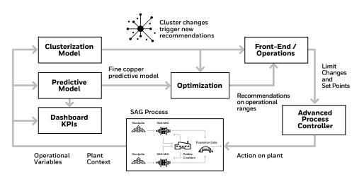
The objective was to maximize the production of fine copper by suggesting actions on the control variables of this equipment. It separated the variables into operational variables, on which we can recommend and act, and those of plant context, including upstream or downstream information, and fed them to predictive machine learning models.
