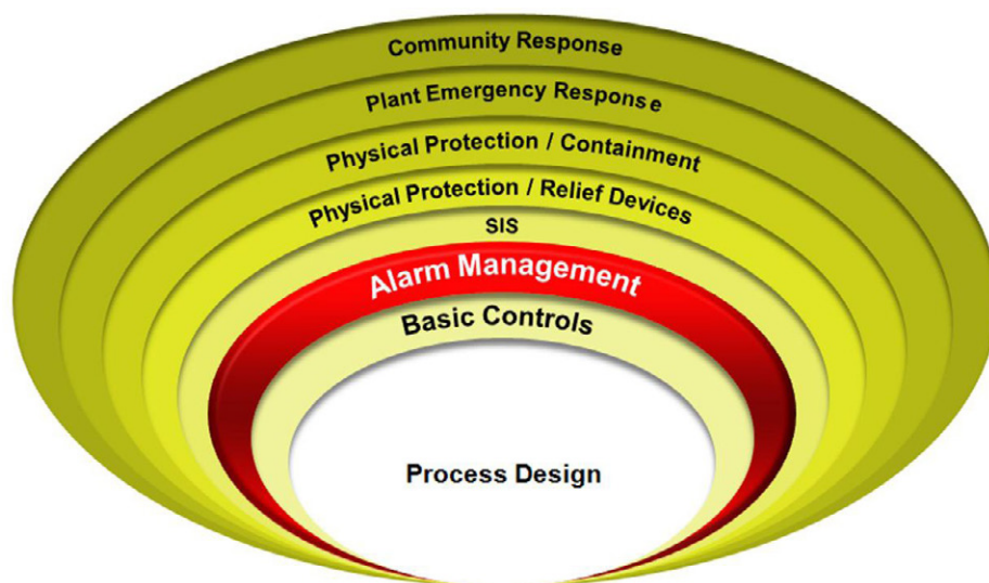
Figure 1: Layers of Protection in a Processing Plant
