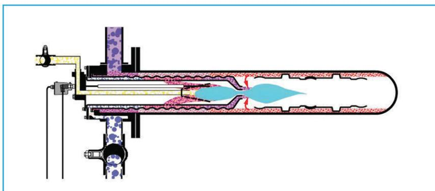
**FIGURE 3.** For applications requiring higher temperatures, one common method to reduce  $\text{NO}_x$  is through the use of flue-gas recirculation (FGR), as shown with the red arrows in this cutaway of a self-recuperative burner in a radiant tube.
