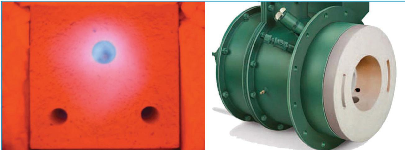
**FIGURE 4.** The telltale sign of a burner designed for staged combustion is an extra set of holes or slots for the secondary stream to travel through and into the combustion chamber. Here, two types of air staging are shown: holes on the left, slots on the right.
