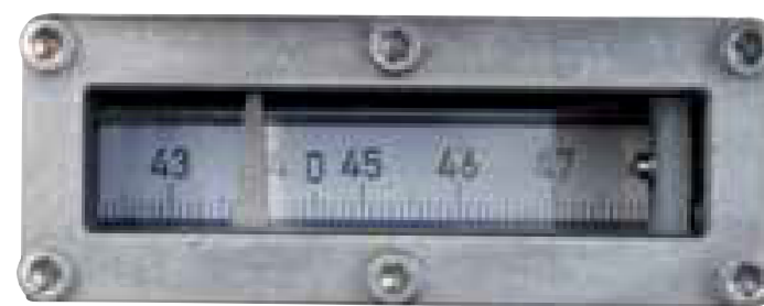
Level reading on graduated tape through window
