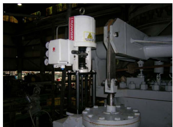
Figure 3. Pneumatic Actuator on pilot operator power cylinder
