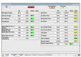
MD control displays clearly present the most important process and control status information to paper machine operators. Actions such as entering set points, changing supervisory control modes, or changing grades, are efficiently performed with a minimum number of steps.
