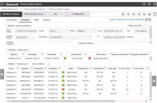
For captured shutdowns inspect details of causes, expected and timely detected effects, and more.
