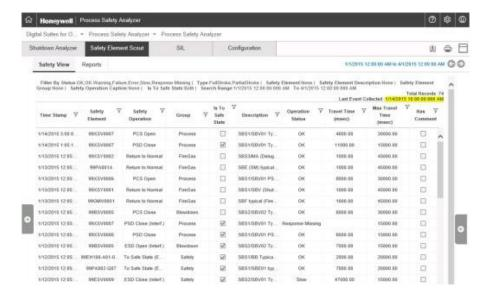
All operations from final elements are captured and validated with details including calculated vs. expected travel time.
