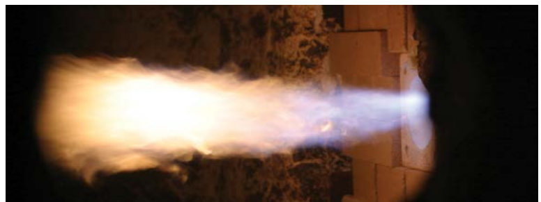
Figure 2: Oxy-Therm LE staged oxygen, conical flame burner.
