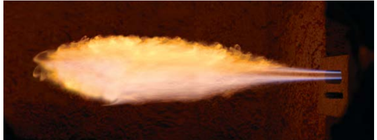
Figure 1: Oxy-Therm FHR adjustable staged oxygen, flat flame burner.
