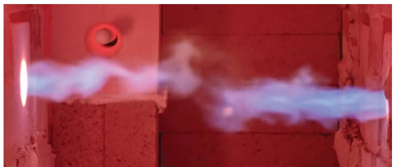
Figure 4: The latest Primefire FH forehearth technology (front right) versus the old technology (rear left).
