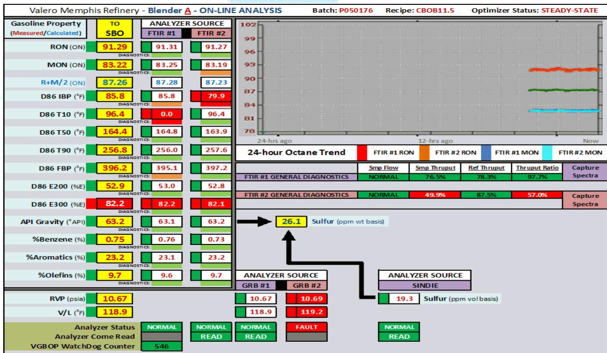
**Figure 3** Spectroscopic Analyzer Diagnostics Control System Graphic
