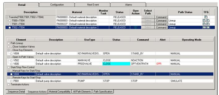
The Sequence Actions tab of the Task Detail display shows the list of actions for a particular sequence for review by the operator
