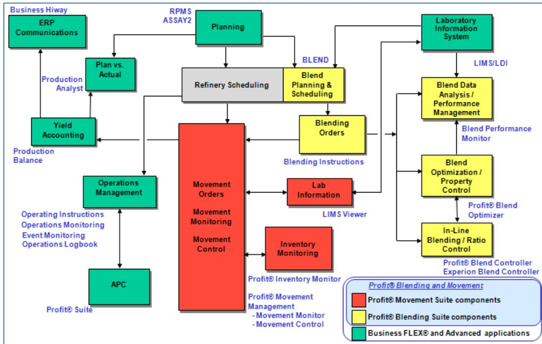
Movement Control is a key component of Honeywell's Profit® Movement Suite and integrates with other Honeywell applications
