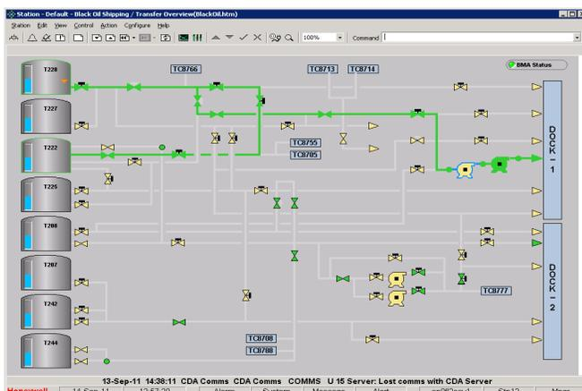
Movement Control uses Tank Farm Graphic (TFG) displays to set up, execute and monitor material movements
