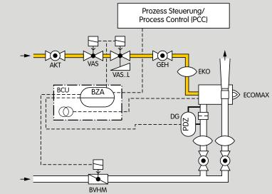
Self recuperative burners are controlled by a rotary impulse system in staged ON/OFF control mode. A variable gas/air ratio control is used to control the gas/air ratio. Alternatively, the air flow can be monitored by a pressure switch.
