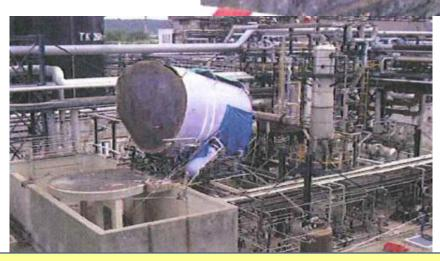
2 workers wounded by explosion of sulphuric acid tank in which hydrogen had formed by adding water
