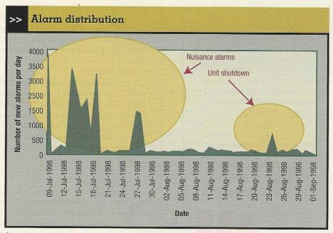
Over-alarming leads to nuisance alarms predominating at sites, which can desensitize operators to alarms that indicate truly serious situations.
