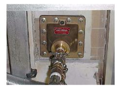
OXY-THERM<sup>®</sup> LE mounted on a glass furnace
