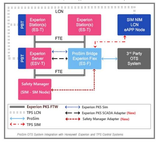
With the ProSim Bridge Enhancement, the SIM-SM and SCADA Adapters may now replace the SM and SCADA emulations, enabling the capabilities of adapters. Here are the key benefits of this enhancement:
