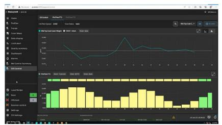
Proven and robust actuator technology combined with market-leading gauging and control solutions by Honeywell guarantees maximal production performance in terms of quality and efficiency. Model predictive CD optimizer allows one coordinated framework for multi-profile control on processes like electrode coating with unusual long time delays. Recipeassociated setpoint database enables operator to save and restore optimal die lip shapes repeatedly just in seconds
