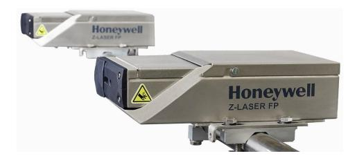
The model 4282 Fixed-Point Rubber Thickness Measurement uses laser triangulation and induction to provide tire manufacturers a non-contacting measurement of the thickness of a rubber sheet prior to being calendered.
