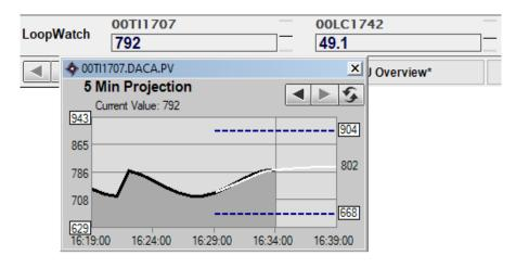
Additionally, ALTIUS 5.8 provides simplified and immediate access to ALTIUS Faceplate Enhancement changes. With 5.8, dynamic changes between all three Keypad Enhancement options as well as the Trend and Averages Faceplate Enhancements are now possible.
