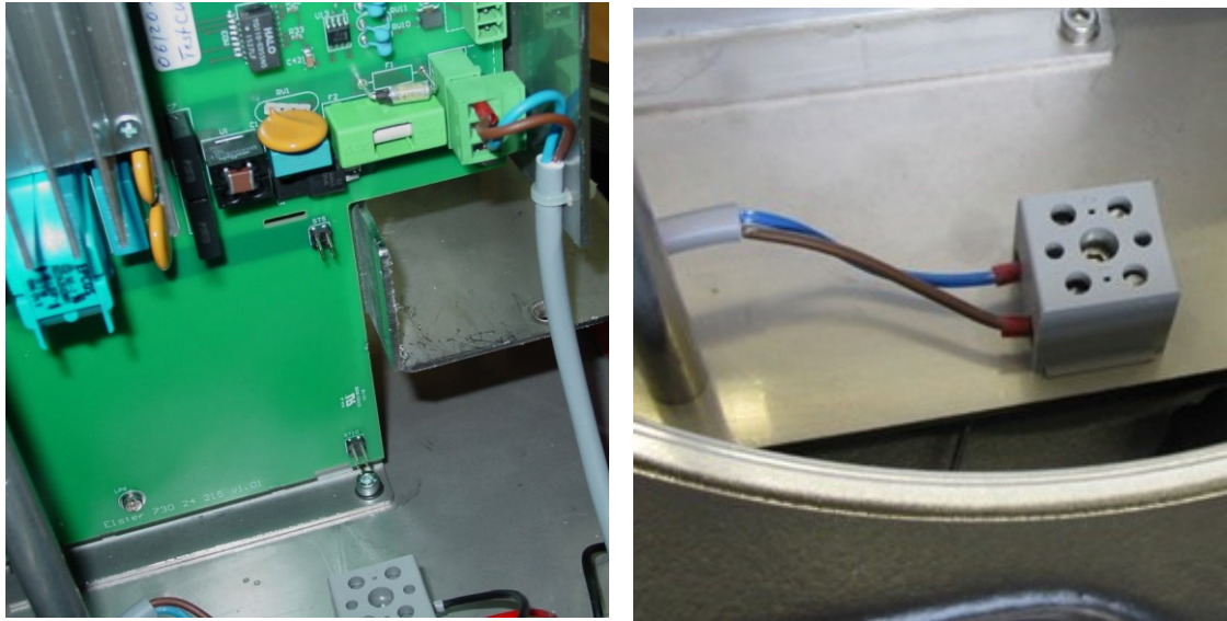
Figure 2.25: Power connection position and details
