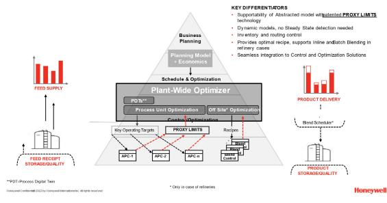
streams can be merged or spitted (or blended in a refinery) to feed the downstream operations. For each unit, a dynamic yield-property model is specified to describe the input-output yield-property relationship. The flowsheet model will then incorporate all unit-level yield-property models to form a global, dynamic hybrid model for online use, similar to the way standard APC models are used online.
