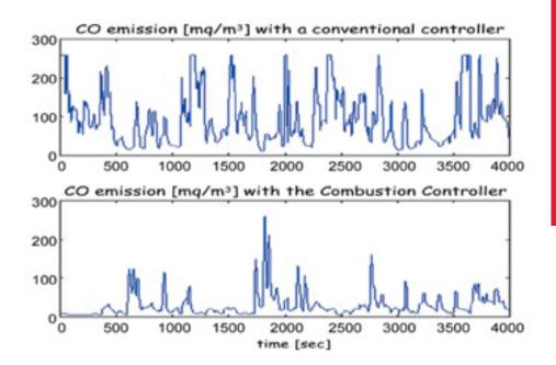
While the example here is a boiler, the benefits of APC can be realized across a wide range of equipment and units in a process plant.
