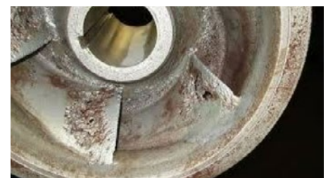
Figure 16: Centrifugal pump blade erosion [Ref: 9.g]
