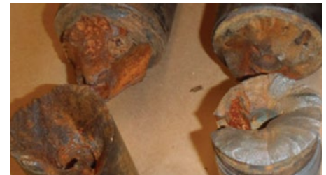
Figure 20: Cracked shaft due to corrosion [Ref: 9.k]
