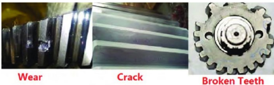
Figure 15: Gear defects [Ref: 9.f]
